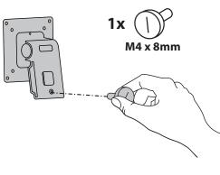
**b** Attach monitors to mounting brackets.
