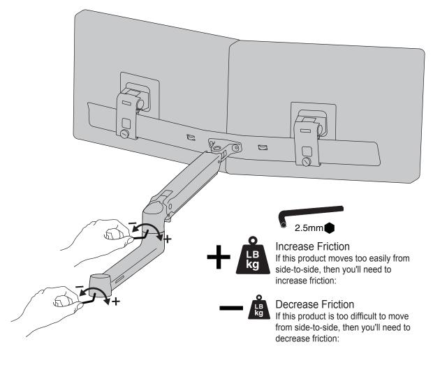
CAUTION: DO NOT remove screw. Removing screw may cause damage to equipment.
